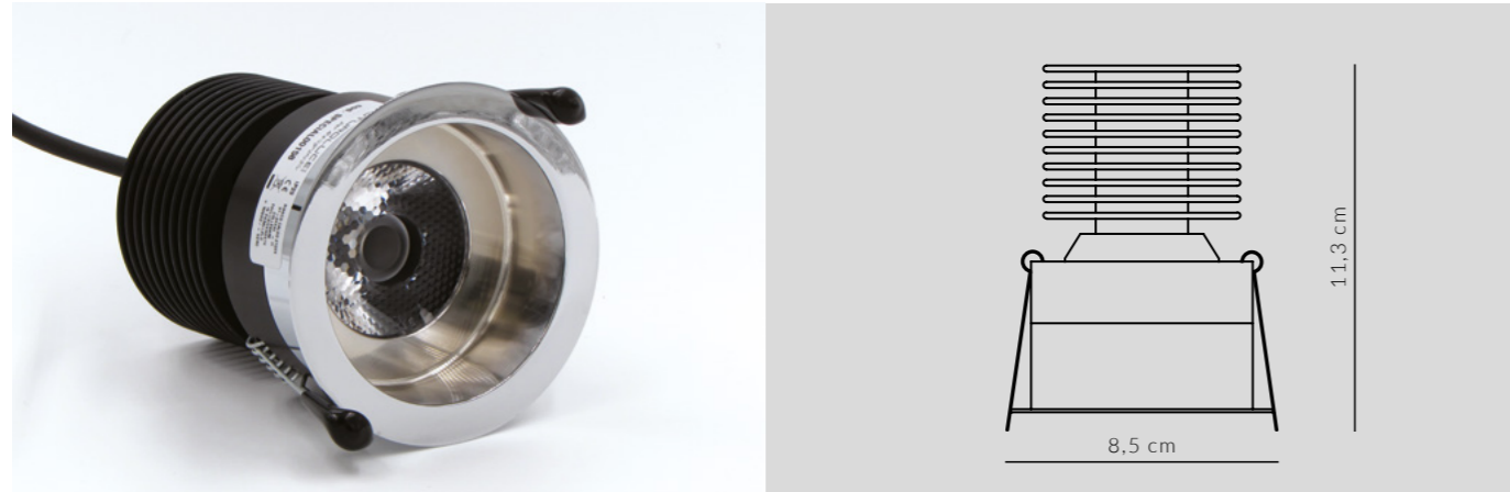
LED recessed projector 10W24Vdc 2700k cri93 optics 6° circular body ø 85 mm.
